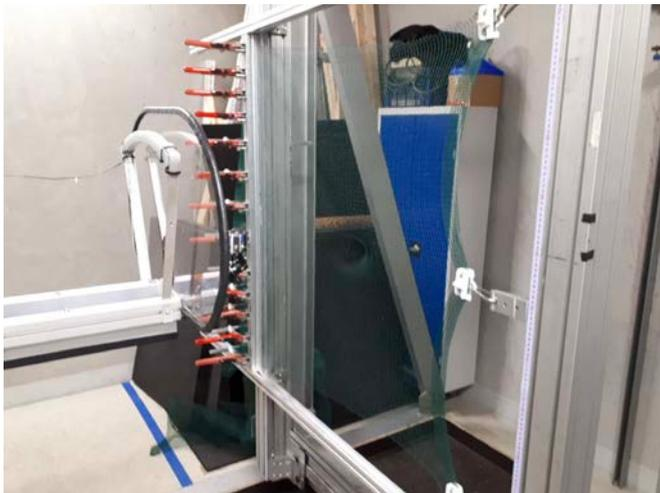
Figure 3: Hail impact cannon in the test laboratory (Source: TÜV Rheinland)
